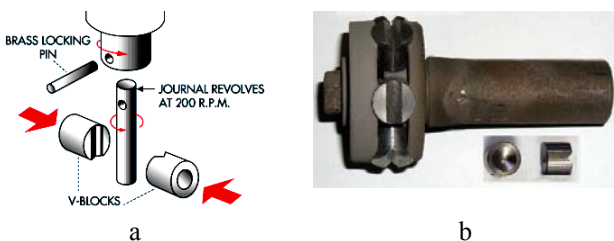
Fig. 2 Principle of the wear test (a) and sample holder for deposition of HVOF coatings (b) [15]
