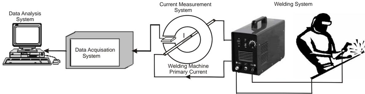
Fig. 2 Measurement system
