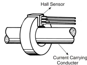
Fig. 1 Current measurement with Hall-effect sensor [12]
