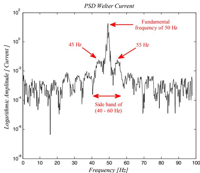
Fig. 6 PSD of current for electric arc welding
