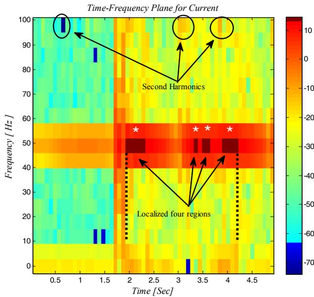
Fig. 5 Filtered Spectrogram (Time-Frequency plane) of the current
