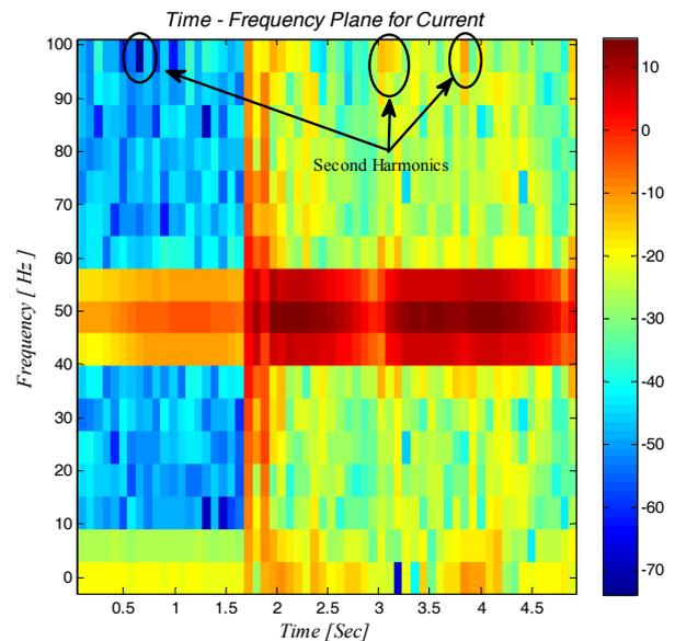
Fig. 4 Spectrogram (Time-Frequency plane) of the current
