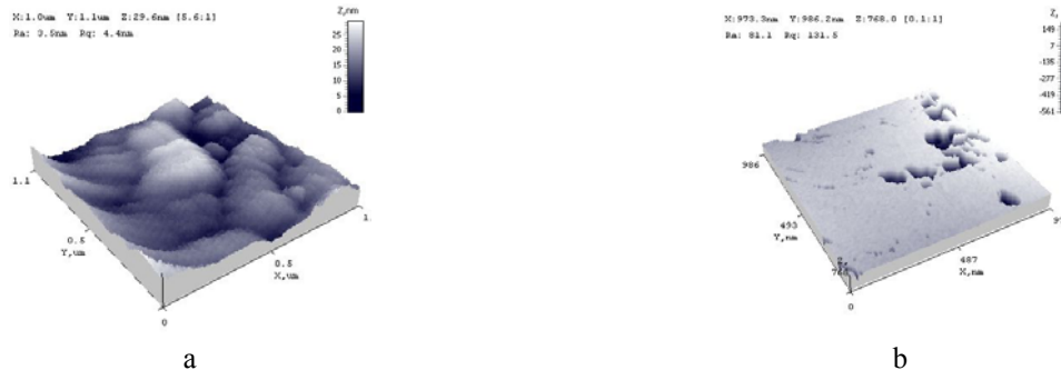
Fig. 4 Lateral force microscopy on PVDF thin films: a - 3D surface morphology of PVDF thin film; b - 3D phase identification of PVDF thin film
