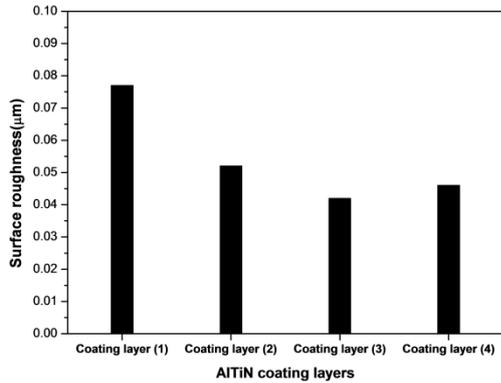
Fig. 3 Surface roughness of AlTiN coating layer measured by AFM
