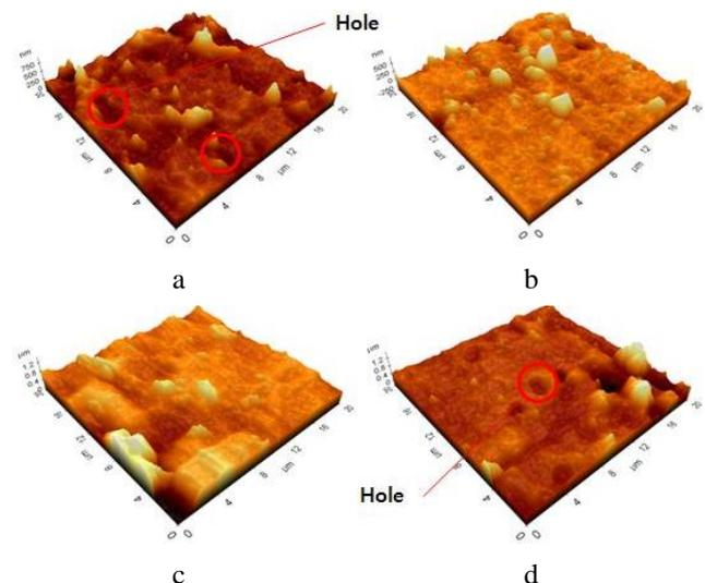
Fig. 2 Surface morphology of AlTiN coating layers by AFM (Scanning 20 $\times$ 20). a - Coating layer (1); b - Coating layer (2); c - Coating layer (3); d - Coating layer (4)
