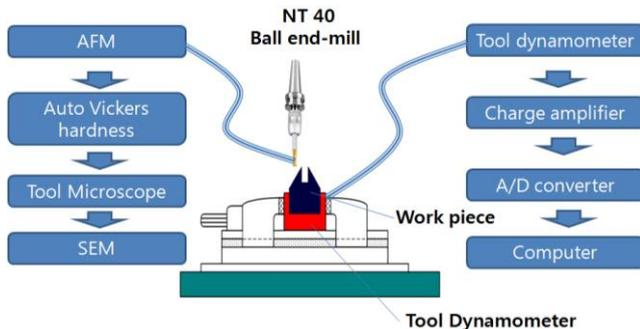
Fig. 1 Schematic diagram of measuring equipment
