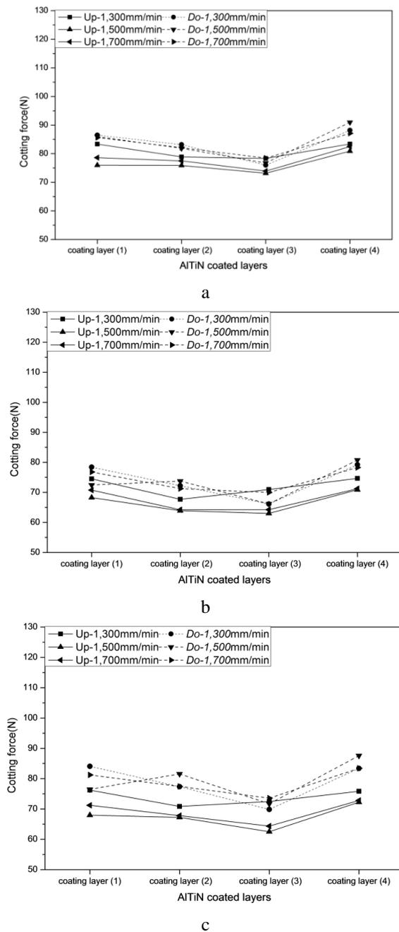
Fig. 6 Three component forces of cutting with the material of inclination according to AlTiN coating layer (d = 0.3 mm, rpm = 10,000). a - Component of forces (Fx); b - Component of forces (Fy); c - Component of forces (Fz)
