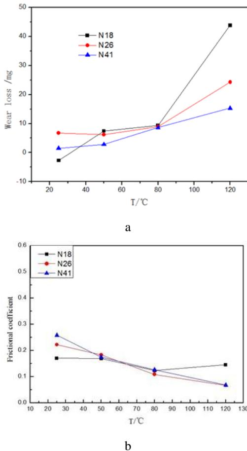
Fig. 6 The wear loss (a) and frictional coefficient (b) of the swelled NBR samples in crude oil at different temperatures
