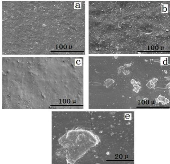
Fig. 3 Surface topography of N26 immersed in crude oil with different temperature for 168 h: a - 25°C; b - 50°C; c - 80°C; d - 120°C; e - 120°C
