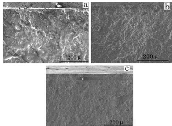
Fig. 5 Tensile failure section morphology of three NBR samples immersed in crude oil at 120°C for 168 h: a - N18; b - N26; c - N41
