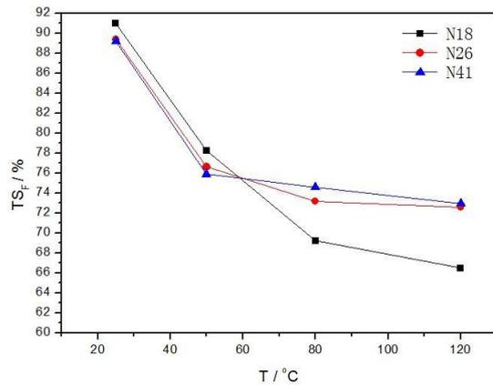
Fig. 4 Variation of tensile strength and tensile fracture permanent deformation at different temperatures
