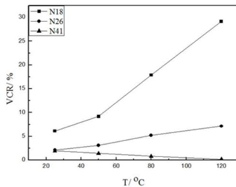
Fig. 2 The effects of temperature on the VCR of NBR
