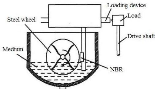
Fig. 1 Schematic of the ring-on-block wear testing machine
