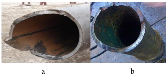
Fig. 1 Broken DPs from rig site: a – fatigue fracture; b – twist-off fracture [5]
