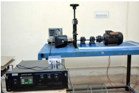
Fig. 2 Bearing test rig setup
