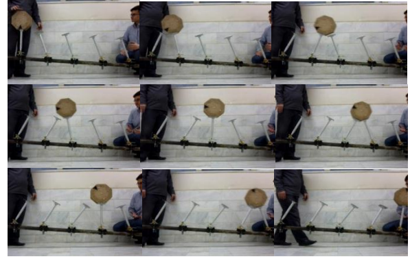
Fig. 6 Experimental implementation of passive manipulation of octagonal object
