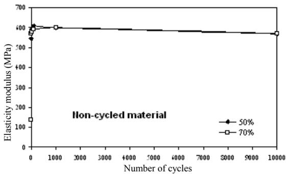
Fig. 7 Elasticity modulus against number cycles (for level of loading 50% and 70%  $\Delta L_{Se}$ )
