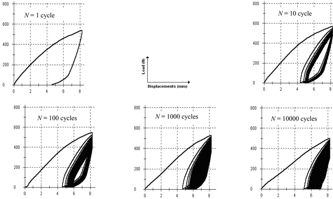
Fig. 5 Load-displacements curves, (for a loading level of 70%  $\Delta L_{Se}$ )
