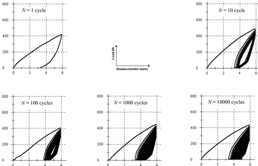
Fig. 4 Load-displacements curves (for a loading level of 50%  $\Delta L_{Se}$ )
