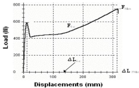
Fig. 3 Load-displacements curve (for  $v = 10$  mm/min)
