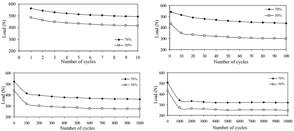
Fig. 6 Cyclic loadings against the number of cycles, (for level of loading 50% and 70%  $\Delta L_{Se}$ )
