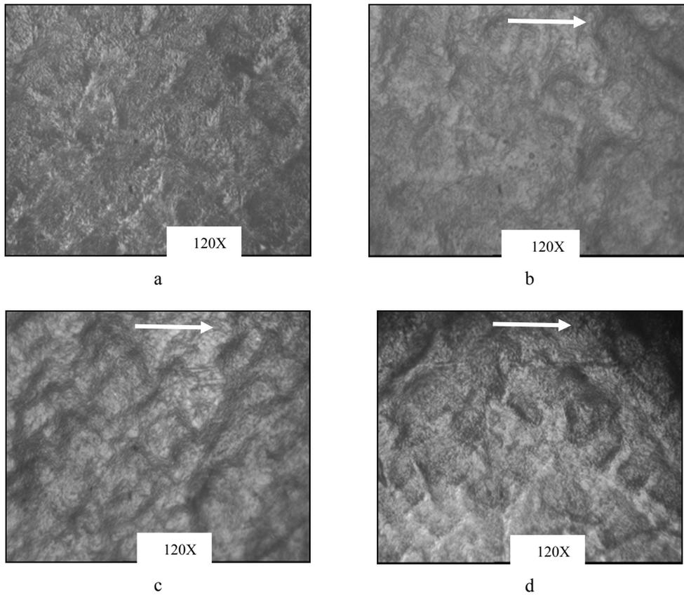
Fig. 8 Structures of the PEHD 80: (a) noncycled, (b) 1 cycle, (c) 100 cycles and (d) 1000 cycles (for loading level of  $50\% \Delta L_{se}$ )
