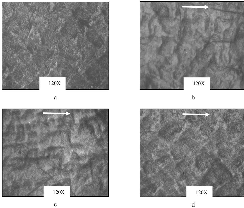
Fig. 9 Structures of the PEHD 80 (a) noncycled, (b) 1 cycle, (c) 100 cycles and (d) 1000 cycles (for loading level of  $70\% \Delta L_{se}$ )
