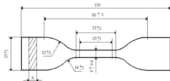
Fig. 2 Detailed dimensions of the sample
