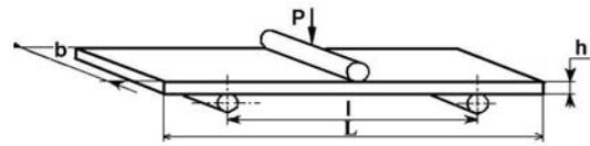
Fig. 1 Three points bending tests set-up
