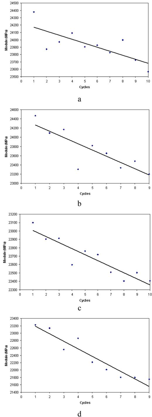
Fig. 4 Modulus by step of load as the function of cycles number: a - loading of material 1, b - unloading of material 1, c - loading of material 2, b - unloading of material 2
