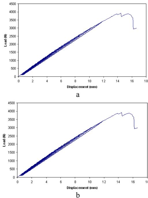
Fig. 3 Load, unload – displacement curves: a - material 1, b - material 2
