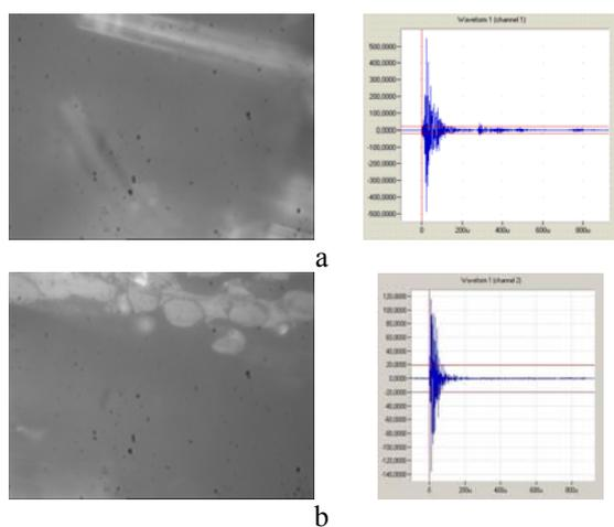
Fig. 9 Mechanisms of damage and rupture in cyclic bending of material 2: a - rupture of fibres extended to  $0^\circ$ , b - interfolds delamination
