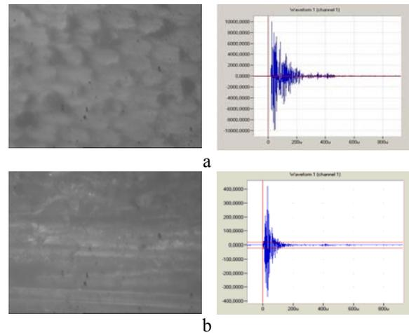
Fig. 6 Mechanisms of damage and rupture in static bending of the material 1: a - interface rupture, b - interfolds rupture
