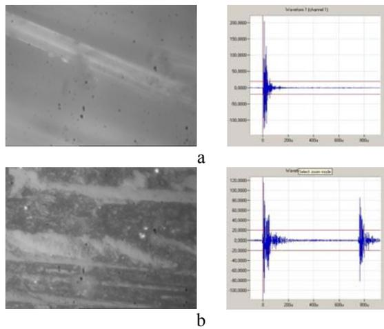
Fig. 8 Mechanisms of damage and rupture in static bending of material 2: a - rupture of fibres extended to  $0^\circ$ , b - interfolds delamination
