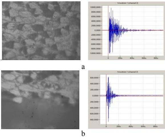
Fig. 7 Mechanisms of damage and rupture in cyclic bending of the material 1: a - interface rupture, b - interfolds delamination
