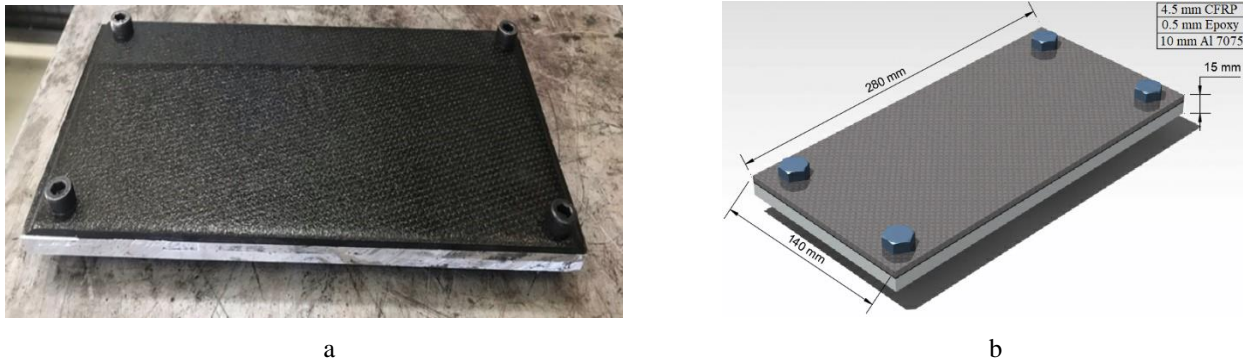
Fig. 1 CFRP/Al 7075 Stacks Material: a - specimen; b - geometry of specimen
