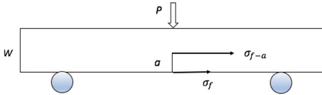
Fig. 2 Schematic view of TPB test specimen
