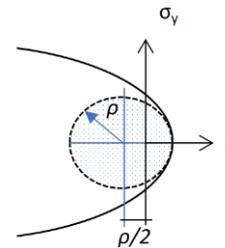
Fig. 1 Stress field coordinate system at hyperbolic notch tip [14]
