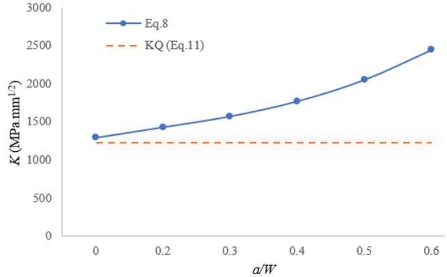
Fig. 6 The increasing mode of  $K_I$  due to pin-loaded geometric factor  $Y$  in the clamped-end condition
