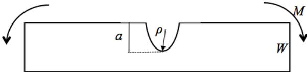
Fig. 3 Bending of a thin beam element [15]
