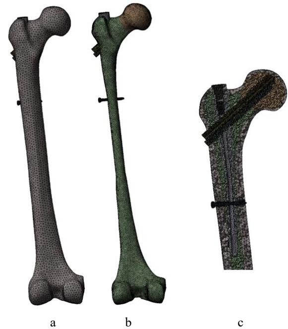
Fig. 13 Screws contact modelling: a – surface-meshed femur geometry, b – assembled femur-PFN model including all implant components, c – cross-sectional view of the implanted femur
