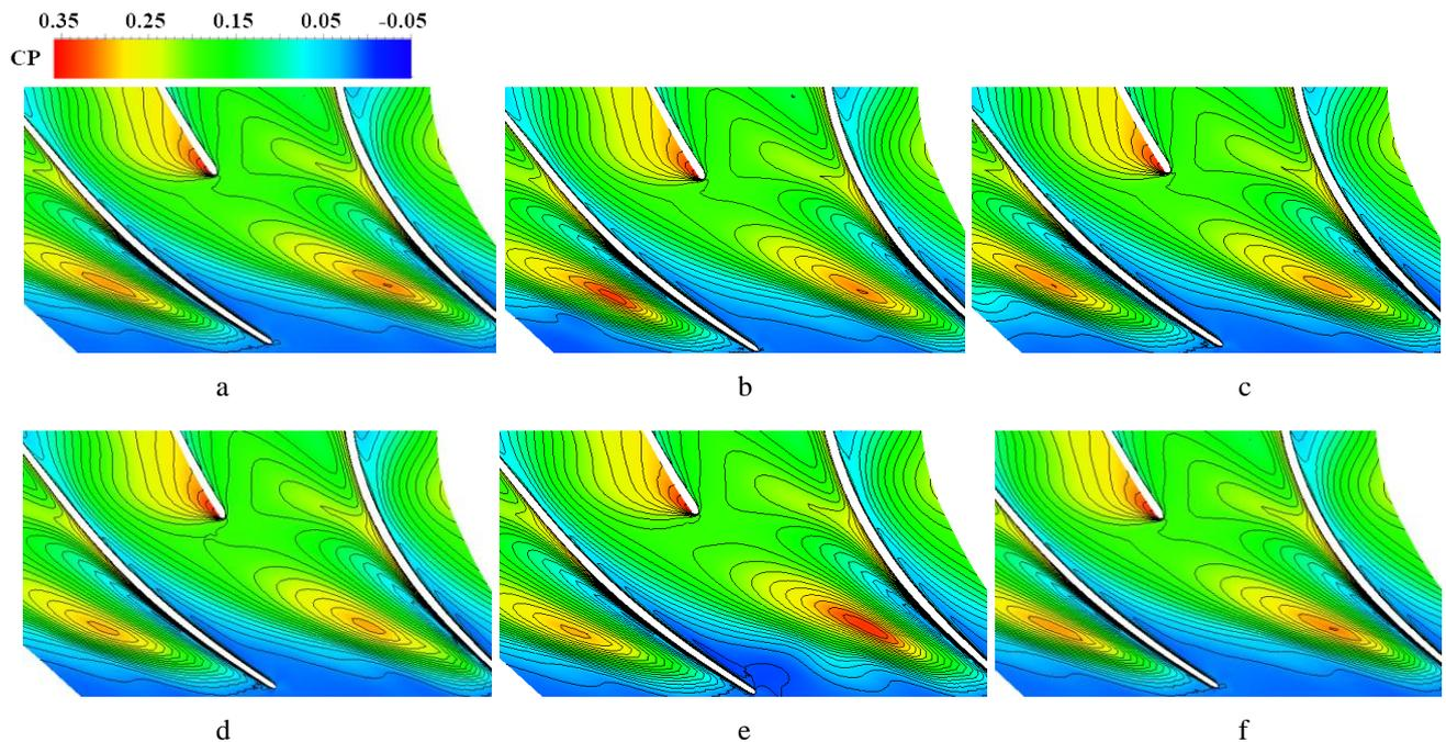
Fig. 5 Transient static pressure distributions at 95% blade height in the case of HC (hole control) operation: a – start point of the period marked as T0; b – 1/5 period, marked as T1; c – 2/5 period, marked as T2; d – 3/5 period, marked as T3; e – 4/5 period, marked as T4; f – the end of the period, marked as T5 (T5=T0)
