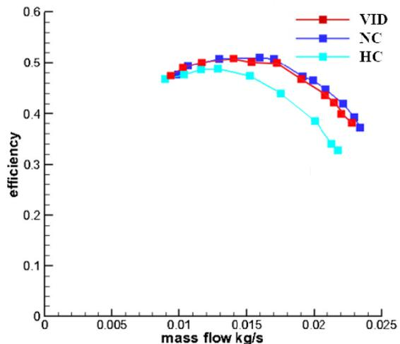
Fig. 12 Efficiency comparison of the micro centrifugal compressor with NC, HC, and VID (NC – no control, HC – with hole control, VID – vortex injection device)
