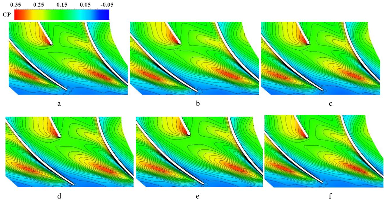
Fig. 4 Transient static pressure distributions at 95% blade height in the case of NC (no control) operation: a – start point of the period, marked as T0; b – 1/5 period, marked as T1; c – 2/5 period, marked as T2; d – 3/5 period, marked as T3; e – 4/5 period, marked as T4; f – the end of the period, marked as T5 (T5=T0)
