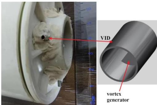
Fig. 9 The tested centrifugal compressor with VID (vortex injection device)
