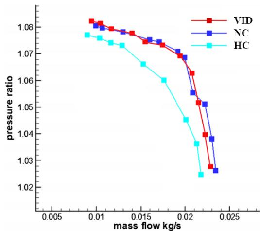
Fig. 11 Total pressure ratio comparison of the micro centrifugal compressor with NC, HC, and VID (NC – no control, HC – with hole control, VID – vortex injection device)
