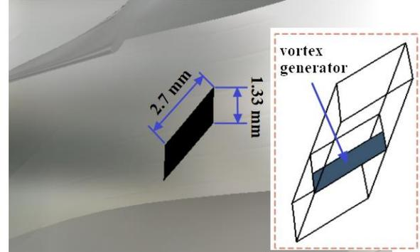
Fig. 1 The sizes of HC and VID (HC – with hole control, VID – vortex injection device)
