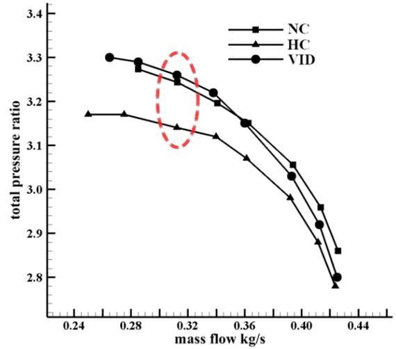
Fig. 2 Compressor total pressure ratio comparison over one blade period (NC – no control, HC – with hole control, VID – vortex injection device)
