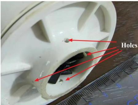
Fig. 8 The tested centrifugal compressor with HC
