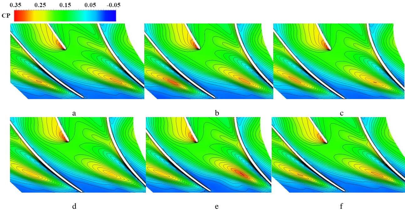
Fig. 6 Transient static pressure distributions at 95% blade height in the case of VID (vortex injection device) operation: a – start point of the period, marked as T0; b – 1/5 period, marked as T1; c – 2/5 period, marked as T2; d – 3/5 period, marked as T3; e – 4/5 period, marked as T4; f – the end of the period, marked as T5 (T5=T0)
