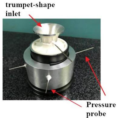
Fig. 10 The assembly of the tested centrifugal compressor with trumpet-shape inlet
