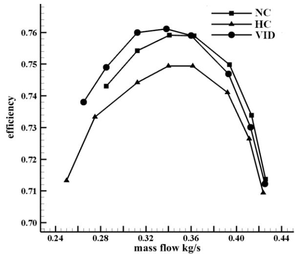
Fig. 3 Compressor efficiency comparison over one blade period (NC – non-control, HC – with hole control, VID – vortex injection device)
