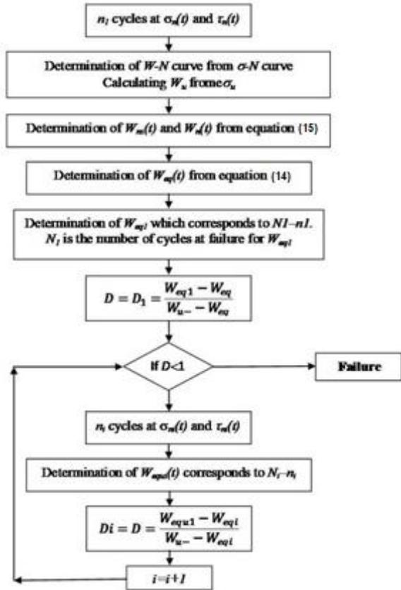
Fig. 3 Algorithm of the damage accumulation and estimation of the life by total strain energy
