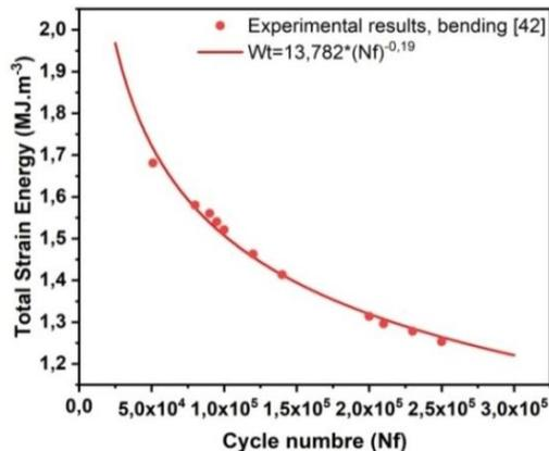
Fig. 5 Cyclic strain energy release rate  $W_i$  versus number of cycles for 30NCD16 steel
