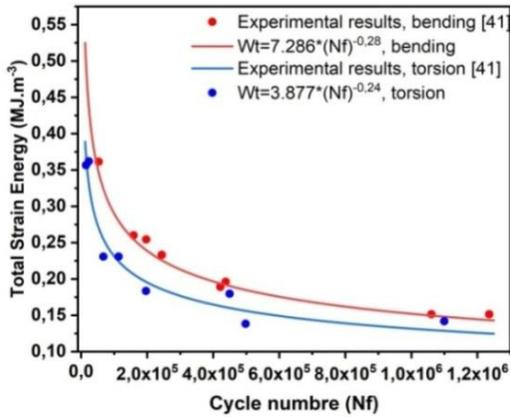
Fig. 4 Cyclic strain energy release rate  $W_i$  versus number of cycles for 6082-T6 Al alloy
