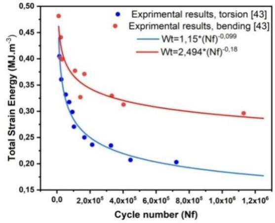
Fig. 6 Cyclic strain energy release rate  $W_i$  versus number of cycles for SM45C steel
