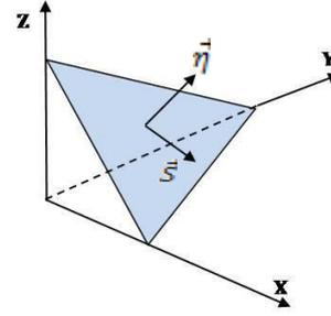
Fig 2 Vector of critical plane in normal  $\vec{\eta}$  and tangential/shear direction  $\vec{s}$
