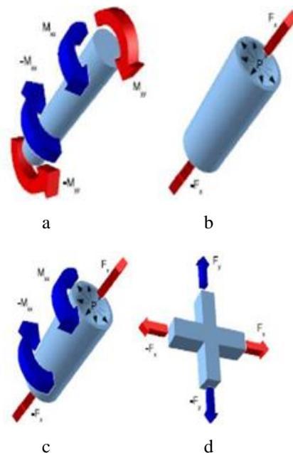
Fig. 1 Types of loading used in multiaxial fatigue: a – torsion-bending, b – tension-internal pressure, c – tension-torsion-internal pressure and d – biaxial tension
