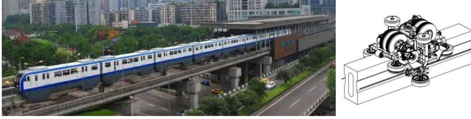
Fig. 1 Chongqing straddle monorail line 3 and its bogie
