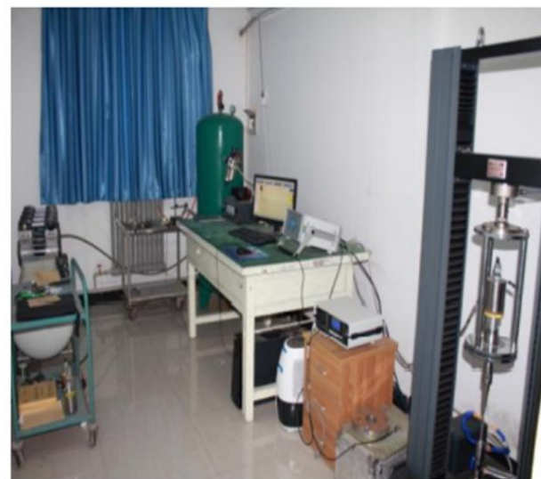
Fig. 4 Fatigue experiment of ultrasonic system: a – schematic diagram of the principle structure, b – picture of the entire system
