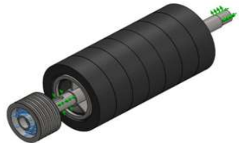
Fig. 20 Modelling and fixation conditions of the decorticator model
