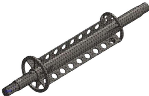
Fig. 38 Meshing on the modified decorticator without abrasive stones
