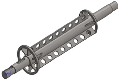
Fig. 36 Modelling of the modified decorticator without abrasive stones
