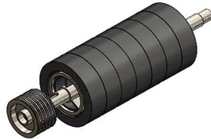
Fig. 19 Modelling the decorticator with abrasive stones using SolidWorks
