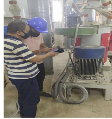
Fig. 6 Operation of vibration measurement sampling on the DHB decorticator
