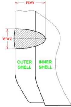
Fig. 2 The diagram shows two-dimension parameters of overlap weld [7]
