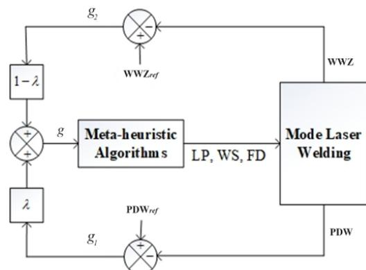
Fig. 1. Diagram of the optimization algorithm
