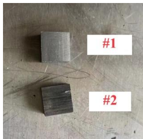
Fig. 5 Two pieces of the as-received crosshead with different wear form
