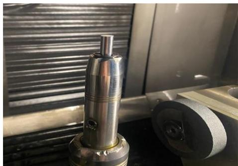
Fig. 1 The appearance of the tungsten carbide sample in the Michael Deckel S22 grinding machine
