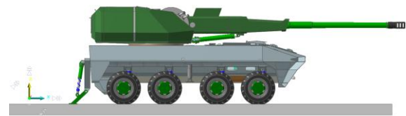
Fig. 15 Dynamic simulation model of the new wheeled artillery based on the vehicle-mounted artillery
