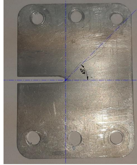
Fig. 10 Example direction of propagation of crack in CTS \alpha = 45^\circ
