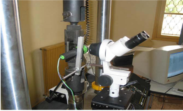
Fig. 4 System (Binocular magnifier – Strobe lamp) used for crack tracking
