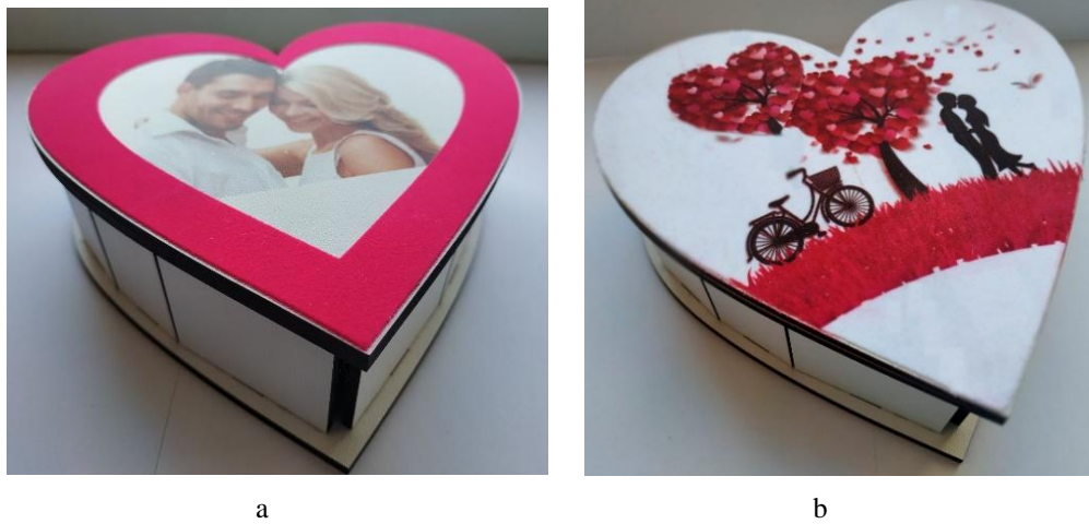
Fig. 7 Image printing and thermal transfer in a thermal press: a – printed image on white flocked material; b – printing on HDF, cutting on a laser engraver and thermal transfer in a thermal press
