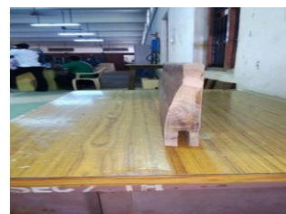
Fig. 4 End of surface showing concave curvature
