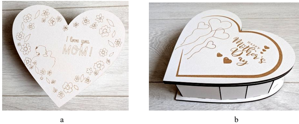
Fig. 6 Laser engraving at a speed of 300 mm/s and power of 40 W: a – contour engraving, b – solid engraving
