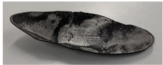
Fig. 9 Example formed part, negative of a knee
