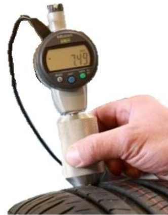
Fig. 4 Tread depth measurement
