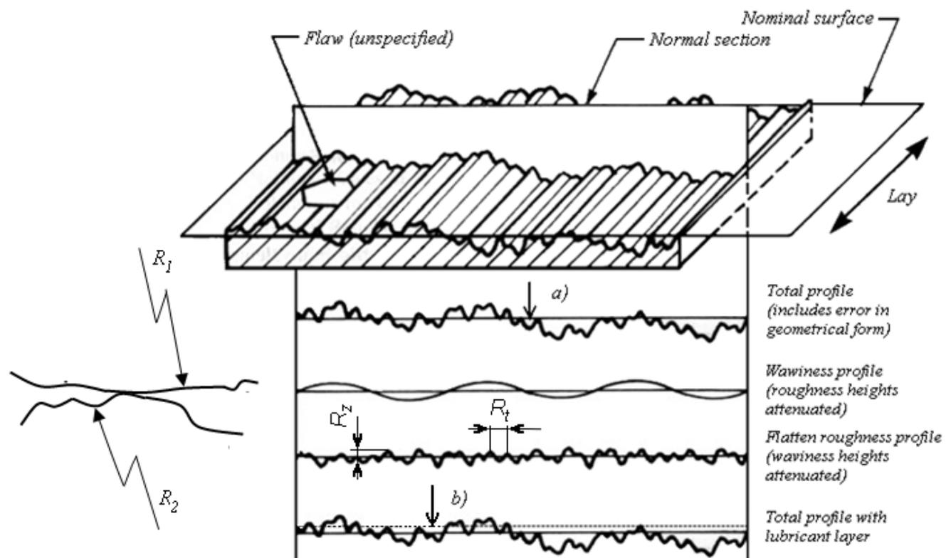
Fig. 1 Model of friction noise generation: a) surface roughness interaction, b) lubricant interference to average roughness pitch and noise frequency,  $R_1$ ,  $R_2$  – radii of contacted surfaces,  $R_r$  – average pitch of surface roughness,  $R_z$  – average height of surface roughness
