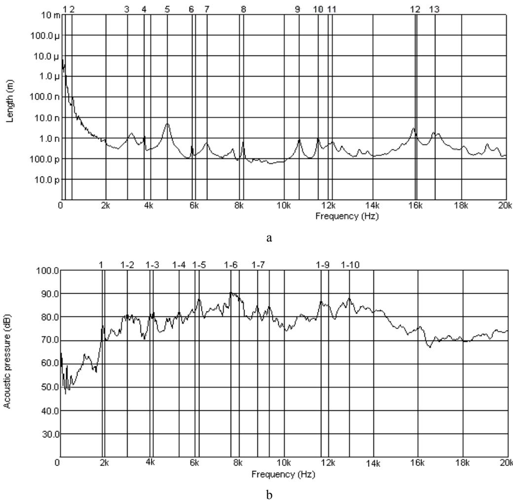
Fig. 8 Vibration amplitude a) and noise b) of ceramic bearing test: material  $\text{Si}_3\text{N}_4\text{-TiN}^9$ ,  $R_a = 0.1$ , 1000 rpm, radial load – 300 N, axial load – 25 N
